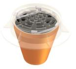
2.2 The FLEXSTORM Inlet Filter frame includes lifting handles in addition to the standard overflow feature. A FLEXSTORM Removal Tool engages the lifting bars or handles to allow manual removal of the assembly without machine assistance. The frame suspension system on most rectangular designs is adjustable in ½" increments up to 5" per side should the casting or drainage structure have imperfections.
