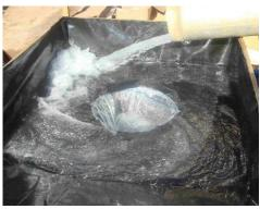
Area Inlet Simulated Showing Influent Discharge From Pipe
